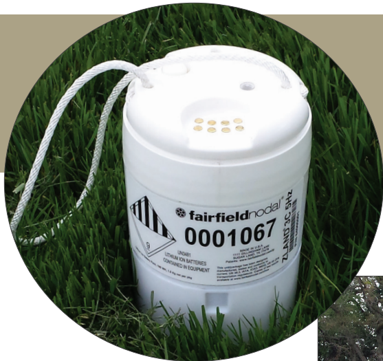
Faculty and students hold a practice deployment of Nodal geophones on the University of Utah campus (below). Closer view of a geophone (inset).
