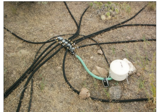
Top: “Spider” of soaker hoses attached to an infrasound microphone at station BRPUi. The hoses act as a type of low-pass filter for the microphone.
