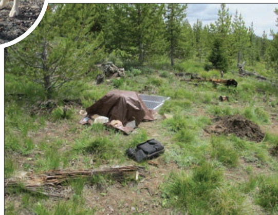
Top left: At station ID01, sensors were buried in buckets. Orange crate was camouflaged with a brown tarp and solar panels laid flat because of low vegetation cover.
