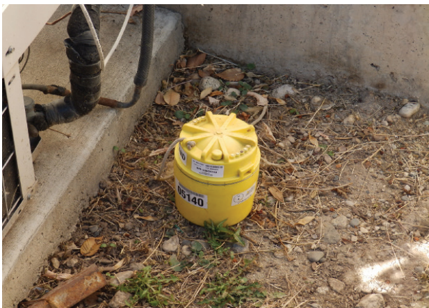
Close-up view of a Nodal Seismic geophone which houses a sensor, datalogger, and a Global Positioning Satellite clock.
