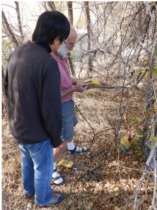
Dr. Fan-Chi Lin looks on as technician Dave Drobeck activates a Nodal Seismic geophone system using a handheld computer.
