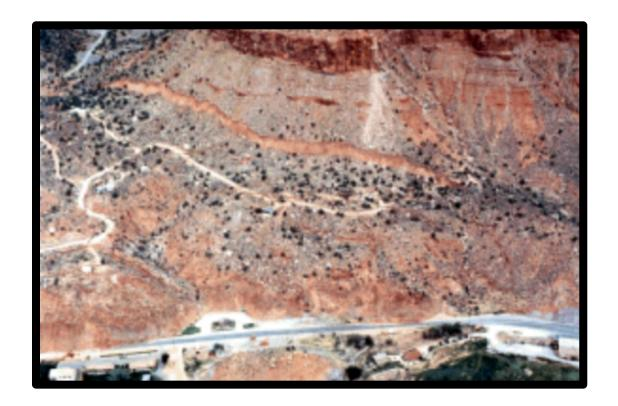
This aerial view to the north of the Balanced Rock Hills Subdivision landslide in Springdale, UT shows the landslide toe covering part of State Route 9 just outside the southwest entrance of Zion National Park. Notice the restaurant that is surrounded, but not touched, by the landslide. Photo by B.J. Solomon, Utah Geological Survey.
