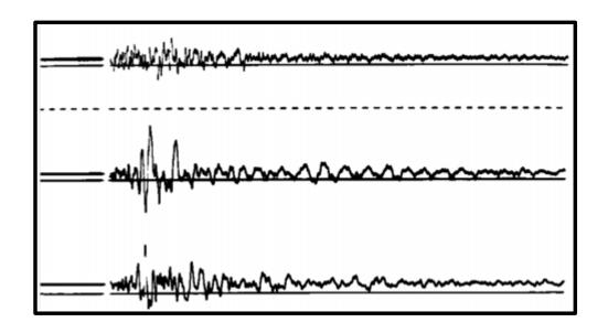
These strong-motion recordings of the vertical (.06g), north-south (.10g), and east-west (.13g) ground accelerations during the Cache Valley earthquake provide engineers with useful data in designing buildings resistant to earthquakes. The instrument itself was owned by the U.S. Coast and Geodetic Survey and located at Utah State University.
