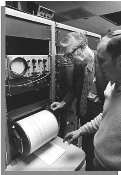
Drs. Kenneth L. Cook (left) and Robert B. Smith (right) examining calibration signals on helicorder in UUSS central recording lab.
